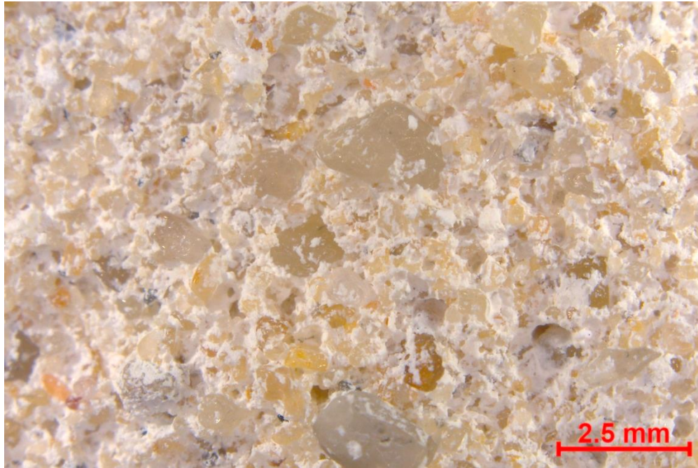
Figure 5. A fracture surface of the stucco showing the uniform paste color and aggregate distribution.
